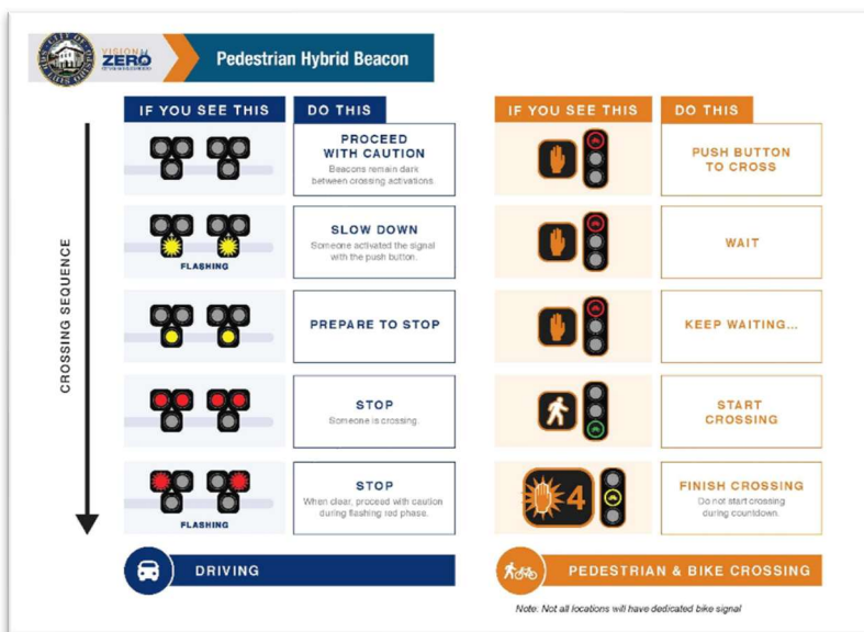
Figure 36 Sequence of a Pedestrian Hybrid Beacon (PHB) 30
